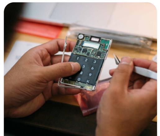
The interior circuitry of a stripped-down Light Phone
